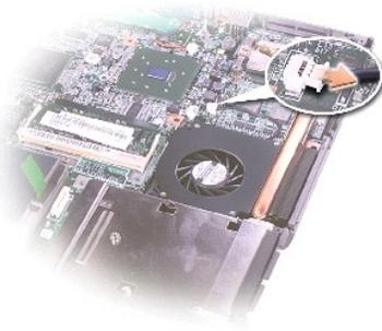
13. Remove the system board from the computer base.
